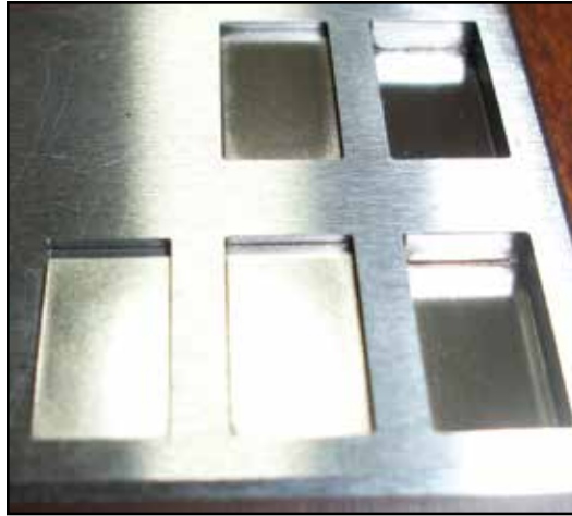
Figure 2: Photo showing fine surface finish available with an appropriate graphite electrode material and proper machine parameters.
